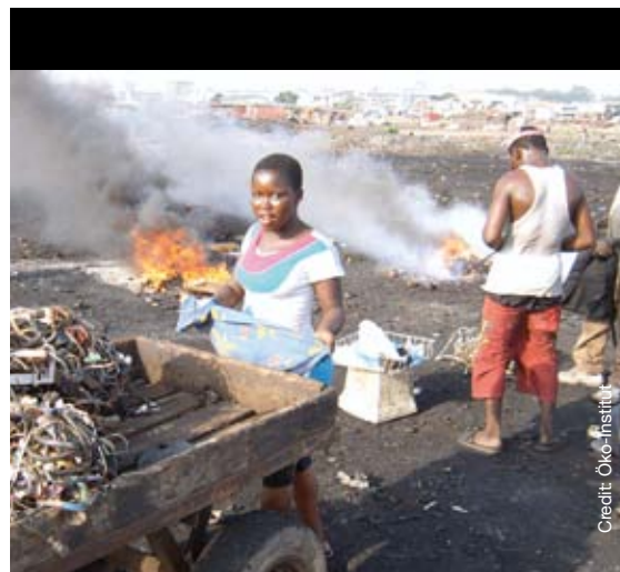
Sorting of cables prior to copper recovery.
