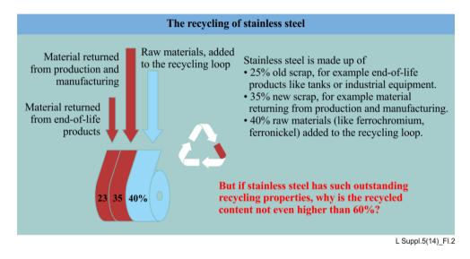
Figure I.2 – The recycling of stainless steel
