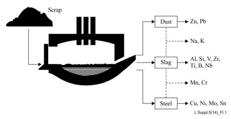
Figure I.1 - Removing impurities from scrap to slag, dust and steel
