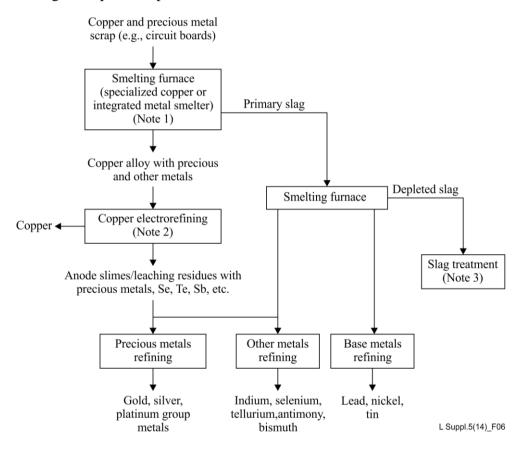
NOTE 1 – Smelters differ in process flow and metals produced. For treatment of materials with plastic content, e.g., circuit boards, special emission pollution control treatment is required for all smelters.
