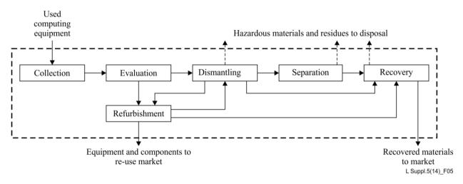
Figure 5 – Flow diagram of environmentally sound management of used computing equipment [b-PACEtrr]
