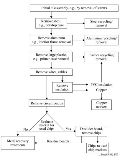
Figure 7 – Manual disassembly and separation of materials
