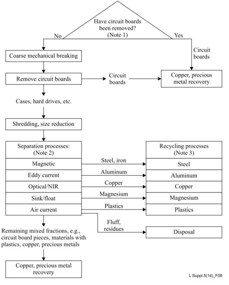
NOTE 1 – Initial removal of circuit boards may be required by national law. If not required, may be removed for economic reasons, to avoid loss of precious metals into other fractions, e.g., steel. NOTE 2 – This is not an exclusive list, and the types and order of separation processes will vary.
