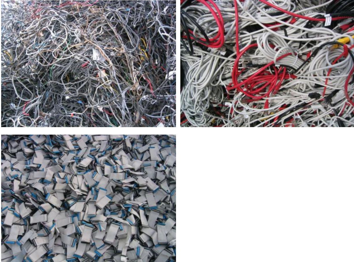
Figure 20: 36 % cable mix 89 (top left) and 12 to 18 % cables from telephone (top right) and connecting cables from PCs (bottom left)
