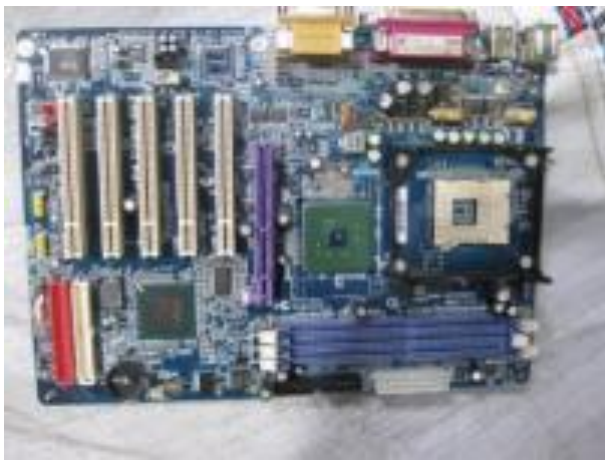
Figure 16: New generation PWB from PCs (Pentium IV and higher)
