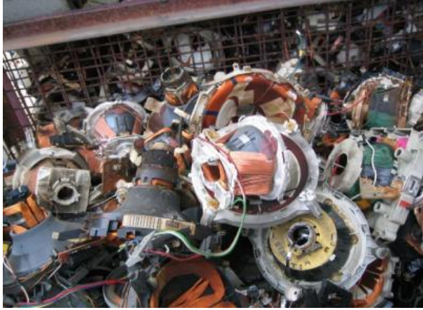
Figure 17: Copper yokes from TVs (left) and power supplies with cables (right)
