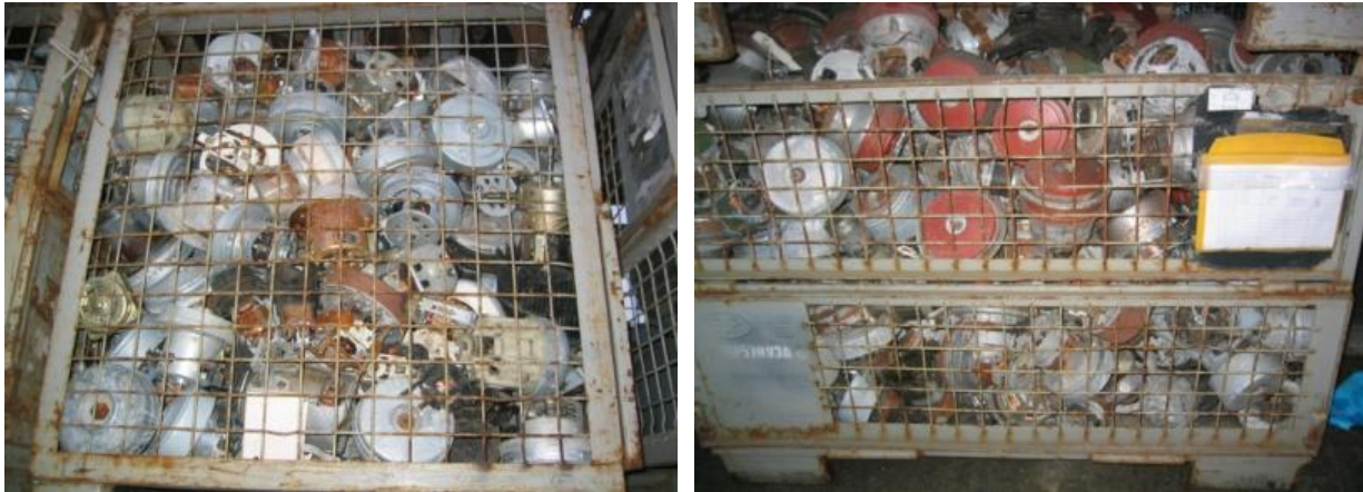
Figure 22: Iron (left) and aluminum motors
